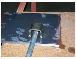
4. Finally, you will want to line up the two holes, and attach them with the bolt.
